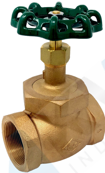
FIG. 109U: CLASS 150 BRONZE GLOBE VALVE NPT ENDS UNION BONNET TEFLON DISC
